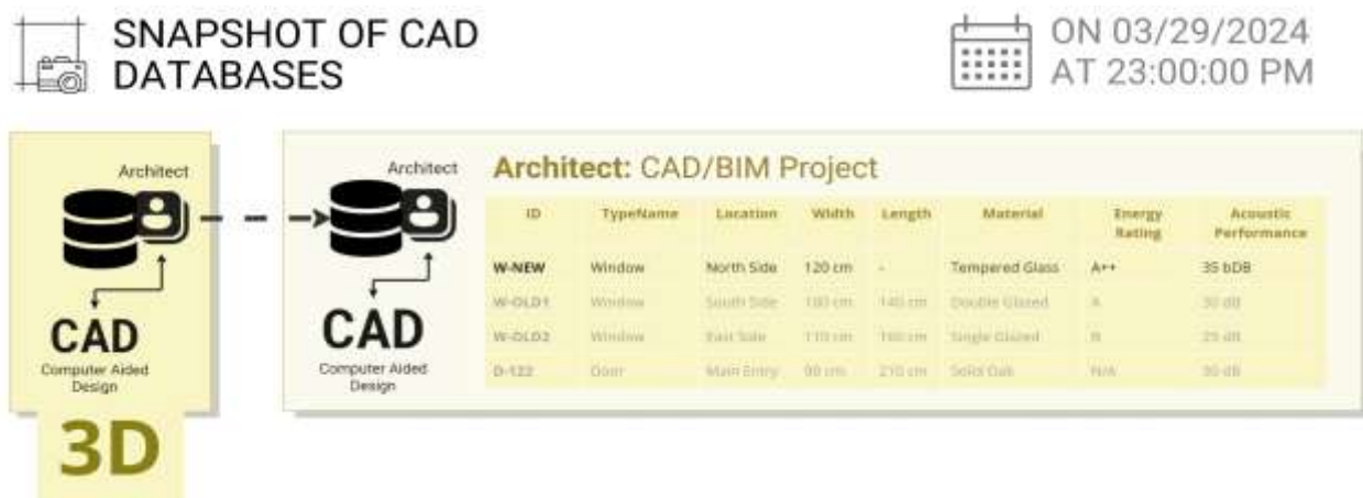
Fig. 4.4-10 CAD database snapshot (BIM) showing the current attribute information for a new entity of class "Window" in the current version of the project model.
