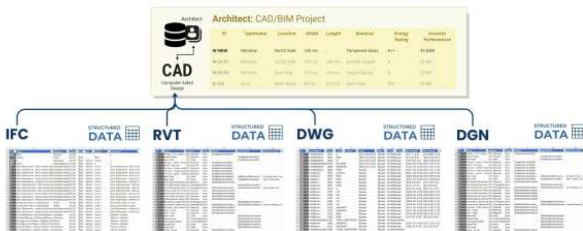
Fig. 4.4-11 Structured data from CAD systems can be a two-dimensional table with columns denoting attributes of elements.
