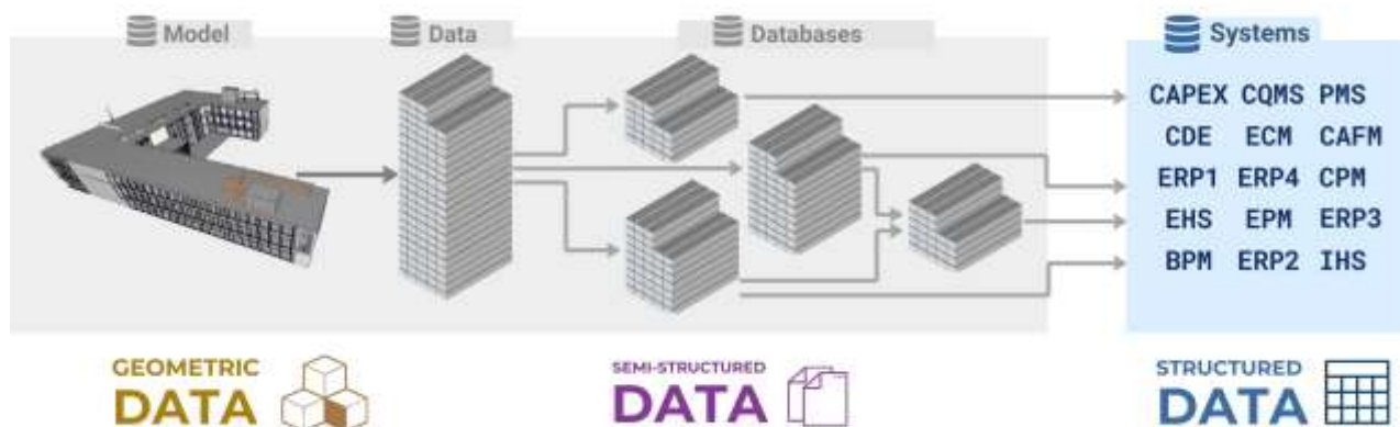
Fig. 3.1-13 CAD tools (BIM) store data in databases that are designed to integrate and interact with other systems.
