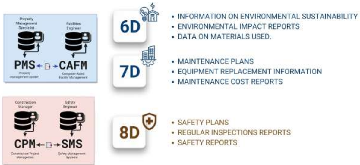
Fig. 5.3-4 Attributes 6D, 7D and 8D in the data information model expand the consideration of various aspects of the project, from energy efficiency to safety.
